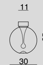
1596.30.1L PLAFONIERA / CEILING LAMP Glass Ø30 H35 cm LED 1 x 12,8W - 350mA - 2700°K or 3000°K CE IP20 Δ 1m
