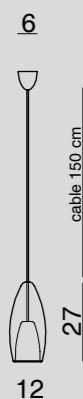
1393.1L SOSPENSIONE / HANGING LAMP Glass Ø12 cm - cavo/cable 150 cm E14 1 x max 60W 220-240V CE IP20 1m
